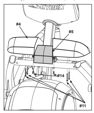
3. Using a Phillips screwdriver, securely fasten the four tap SC 10-12 x 2.00 Type A PN HD PHIL (#11).
