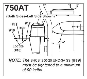
8. Verify the SHCS .250-20 UNC-3A SS (#19) are tightened to a minimum of 90 in/lbs.
