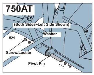
2. Apply loctite (#16) to threads inside the arm and both screws removed in step 2 of **Remove left** and right handle assembly.
