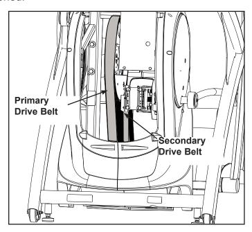
NOTE: If a belt has cracks or appears worn, it must be replaced immediately by a qualified service technician.
